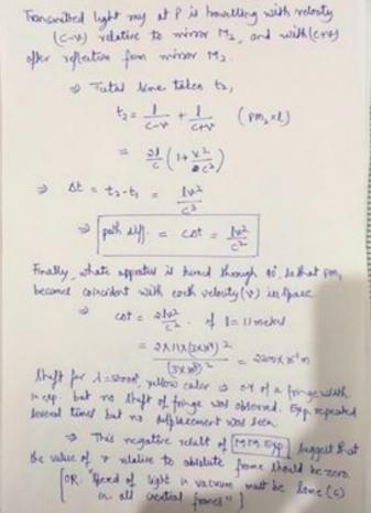
**Note:** The negative result of this experiments suggests that the speed of light In vacuum must be same (c) in all inertial frames.
